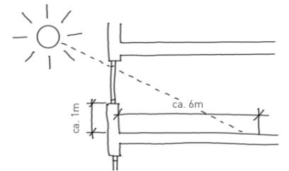
...but avoid unnecessary glazing underneath the usual breastwork height.
