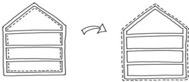
Insulate the building on the exterior to avoid thermal bridges...
